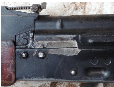
Marking erased on an AKM collected by MISCA
